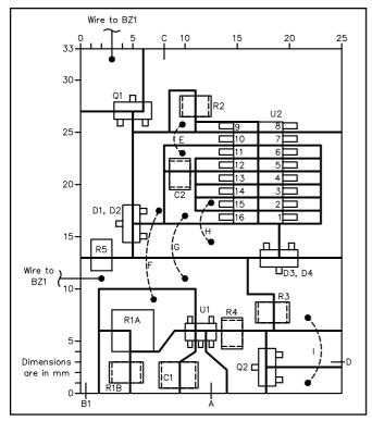
Figure 20—PC board layout of the 10-minute timer. Heavy lines designate cuts made in the foil to create component-mounting islands as described in Part 1 of this series.
